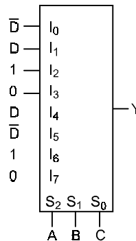
Fig. 4.23 An 8-line to 1-line MUX implementation of a function of 4 variables
